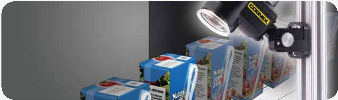
Checker detects a part by finding an actual part feature, such as the apple graphic on top of the juice boxes. This provides extremely reliable part detection, unattainable with photoelectric sensors. The optional SensorView display lets users see exactly what's being inspected, as well as production statistics.
