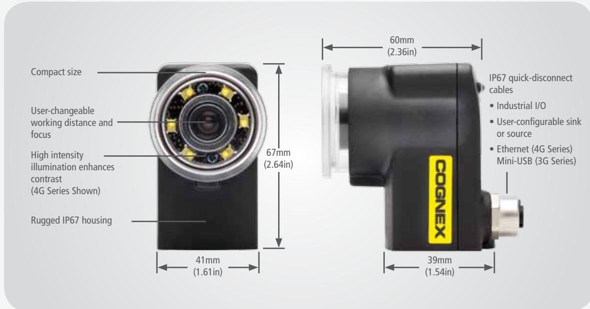
Checker 4G with Ethernet easily integrates into your factory network. From one PC, you can remotely setup and monitor Checker(s) on your network, communicate to your PLC and FTP transfer an unlimited amount of images for storage and/or review.
